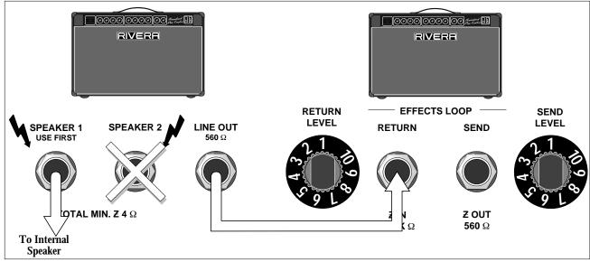
Using a shielded cord, connect the first Hundred Duo Twelve's Line Out to the Effects Loop Return jack on a second Hundred Duo Twelve. Adjusting the Return Level sets the relative volume of the second amp. All tone and distortion adjustments are made by the first amp. Alternatively, you can use the Effects Loop Send jack from the first Hundred Duo Twelve instead of its Line Out. The Send Level control sets the signal level being sent to the second amp.
