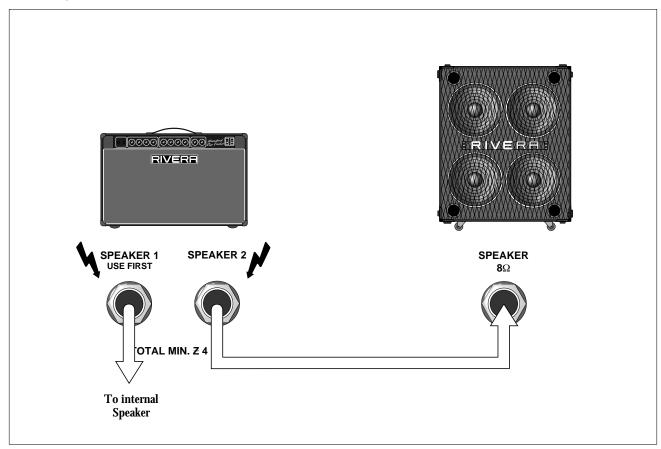
Using a heavy-gauge speaker cord, connect the output jack labeled Speaker 2 to the speaker input on an extension cabinet with a 4- or 8-ohm impedance and power-handling capacity of at least 100 watts. A 16-ohm extension cabinet can also be used, but it will reduce the amp's output. Don't use a 2-ohm extension speaker. Note: Make sure that the Speaker 1 output is connected to the Hundred Duo Twelve's internal speaker.
