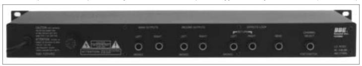
The Model 381's rear panel features stereo main and recording outputs, a mono/stereo effects loop, and a jack for the remote channel selector.
