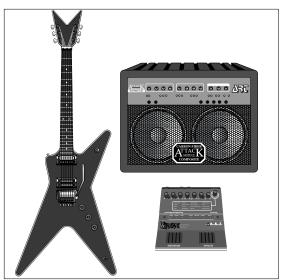
Patch the XTREME into the effects loop of an instrument amplifier as shown (for mono setups, use the XTREME's Output 1 jack). If the amp has two effects-loop return jacks for stereo operation, you may connect a second cord between the XTREME's Output 2 and the amp's second return jack.
